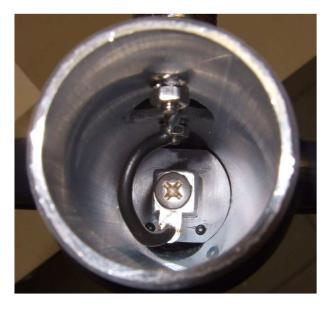
Align the solder tag and tighten the M4 screw. Bend the tag upwards for maximum distance to the center post wall.
