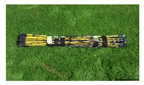
Antenna setup is proceeded in reverse order, of course. Remove the velcro straps step by step, carefully unfold the spreaders and get the wires and cords sorted. Do not tighten the locking swivel joints until all wires and cords are in place.
