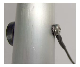
Take the wire to the corresponding wire clip on the spreader top left, and attach to the clip. There should be no or little sag in the wire. Now run the element assembly clockwise along the spreaders and attach to the appropriate clips.
