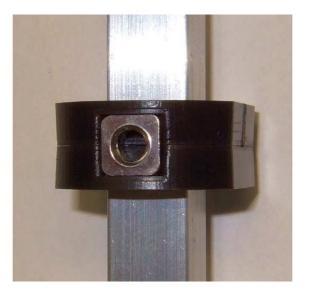
Now carefully insert the center conductor into the center post with the rounded end of the rod facing the top of the center post. Move the rod until you can see the square nut's threads though the small holes, and the threads in the rod through the large holes (and through the centering discs, of course).
