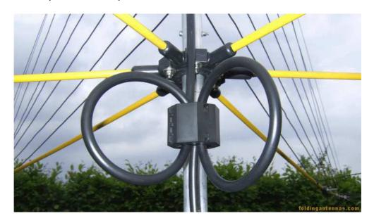
In addition, this core is great as a line isolator for RFI fighting on your neighbour's tv or radio. It easily takes the thickest wires without touching them and is installed in a few seconds.
