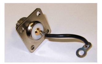
□ Insert a M4 x 8 pan head screw into the solder tag and push a M4 lock washer on the thread from the other side.
