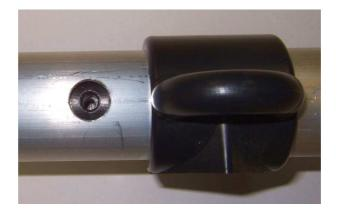
Put a feedthrough insulator on every large hole and secure loosely with a M4 x20 pan head screw. Enlarge the hole in the insulator a tad with a 4 mm or 5/32" drill if required. Insert M4 x 8 pan head screws in all 6 small holes and tighten loosely. The center conductor is now held in position.
